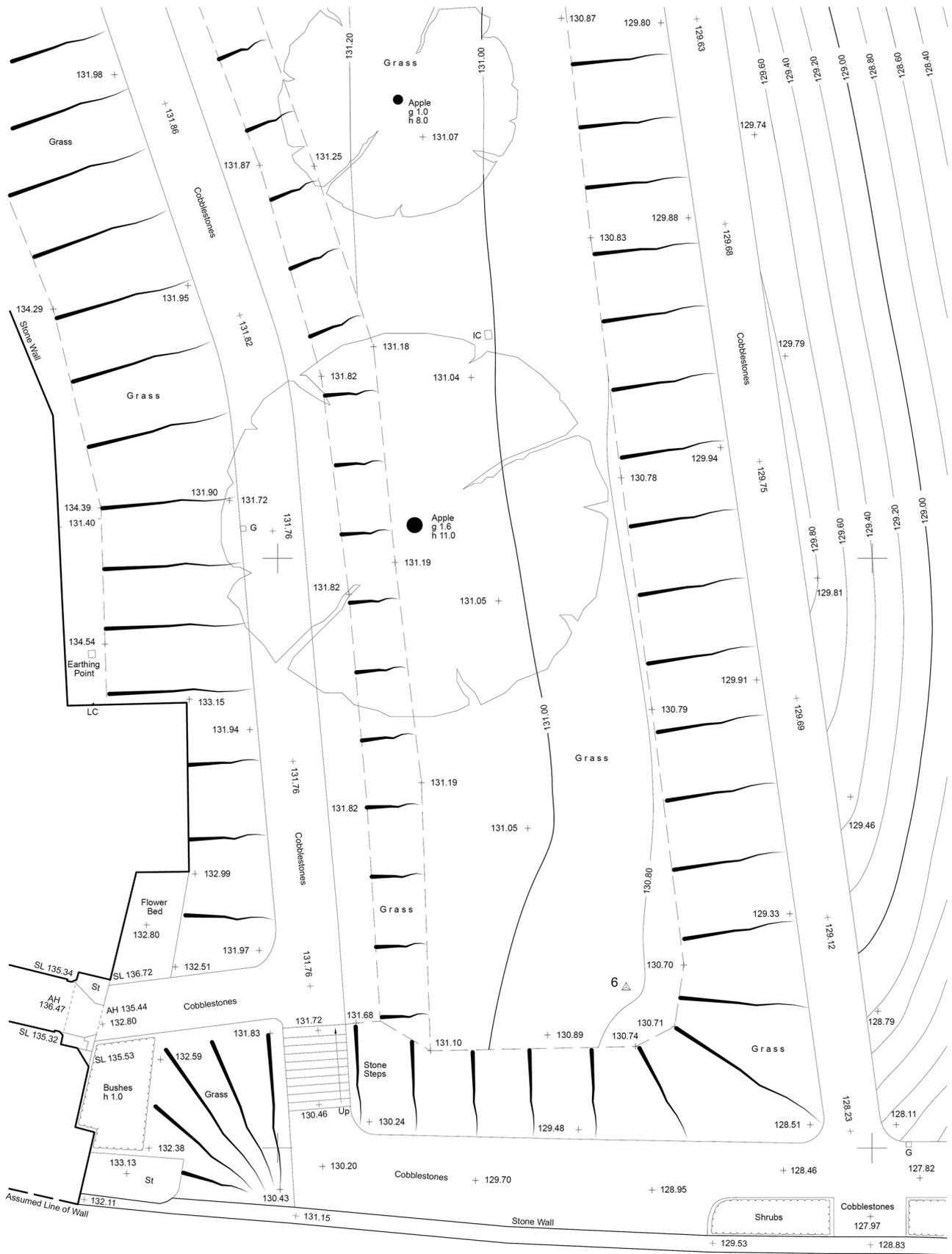
Figure 6.6: Use of hachures to supplement information from contours. Originally prepared for presentation at 1:200 scale.
